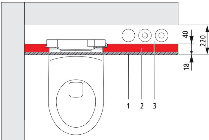
Abb. 23: Optivis-Tec-Vorwand 220 mm
